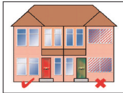
Figure 37: Matching new windows to existing building
