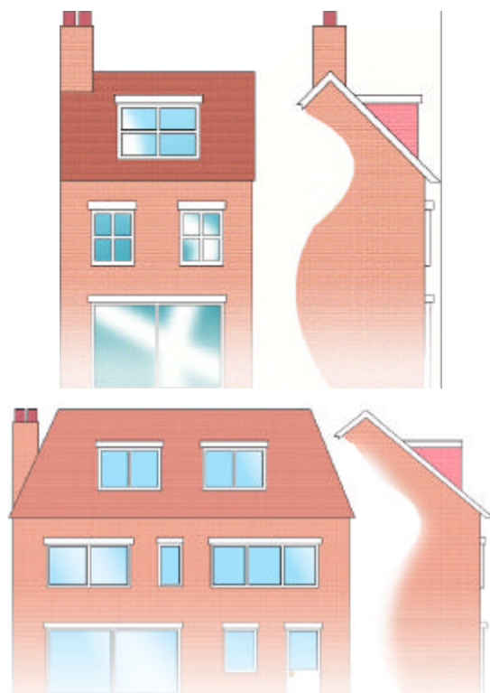
Figure 45: Position of dormer within the roof slope.
