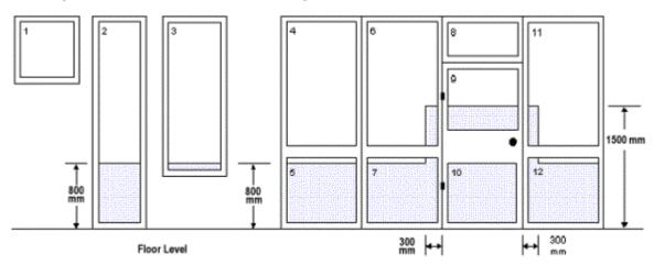
The diagram above gives examples of glazing in windows, partitions, walls, doors and side panels. 'Critical locations' are shaded grey. Any glazing within a shaded area must comply with BS 6206.
