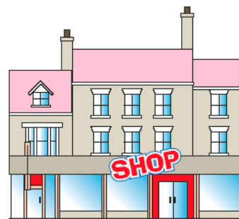
Figure 3: A shop front that does not respect the original building
