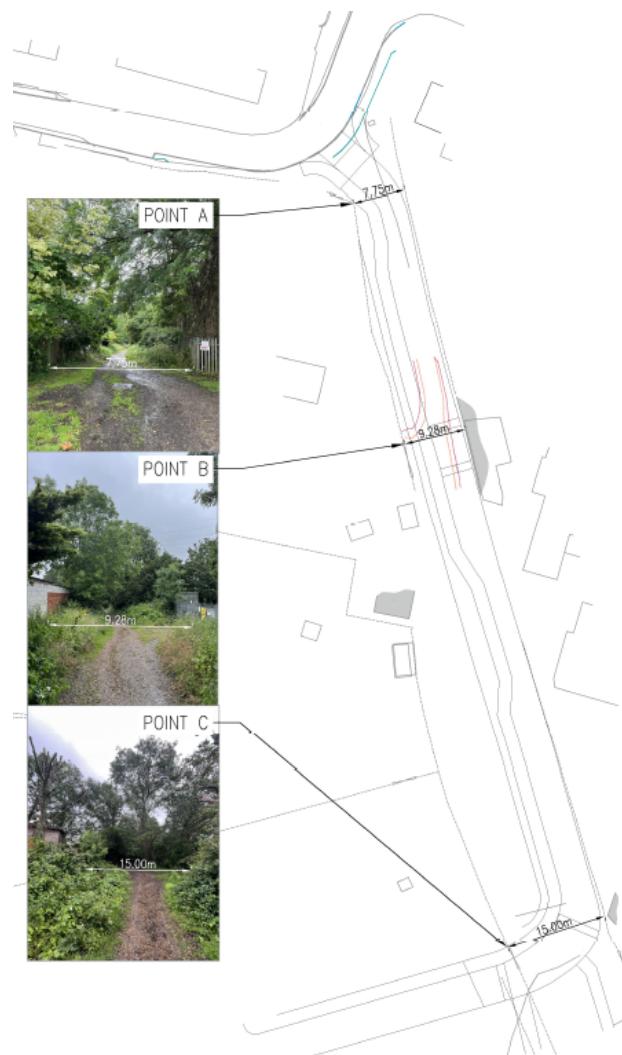
Figure 4 – Access widths with photos
