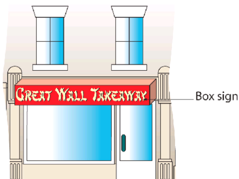
Figure 8: A box sign.
