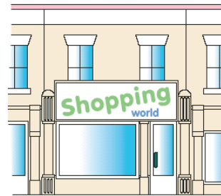
Figure 2: A disproportionate fascia board.
